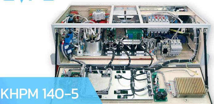
MAIN AND AUXILIARY CONVERTER FOR ELECTRIC VEHICLES
